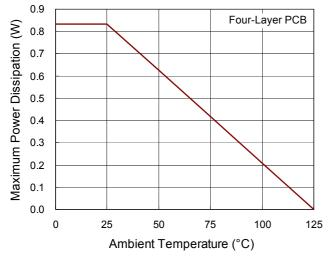
Figure 3. Derating Curve of Maximum Power Dissipation
