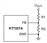
Figure 1. Output Voltage Setting
