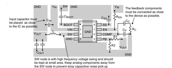
Figure 9. PCB Layout Guide
