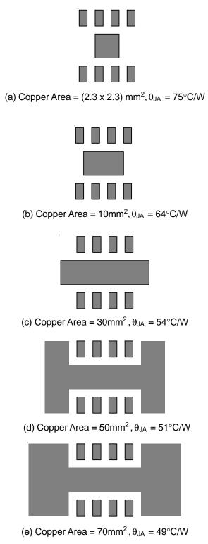
Figure 7. Themal Resistance vs. Copper Area Layout Design
