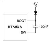
Figure 2. External Bootstrap Diode
