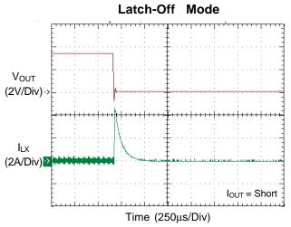
Figure 6. Latch-Off Mode Under Voltage Protection
