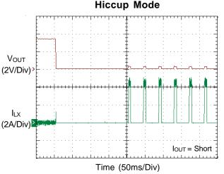
Figure 5. Hiccup Mode Under Voltage Protection
