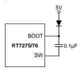
Figure 5. External Bootstrap Diode
