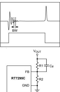
Figure 1. Cff Capacitor Setting
