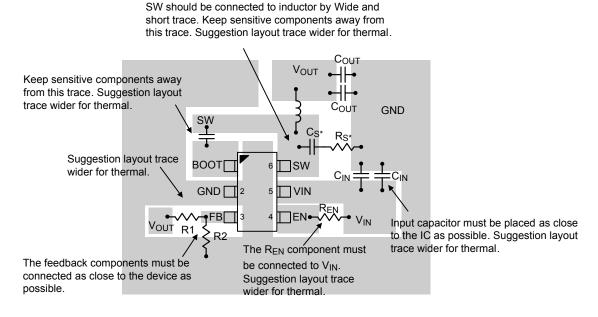
Figure 8. PCB Layout Guide
