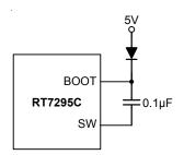
Figure 6. External Bootstrap Diode
