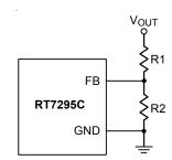
Figure 5. Output Voltage Setting
