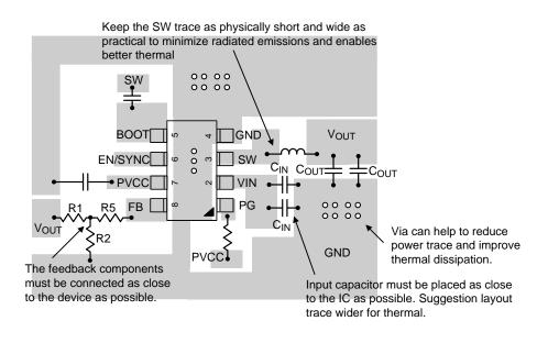
Figure 6. PCB Layout Guide
