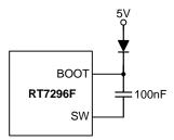
Figure 4. External Bootstrap Diode
