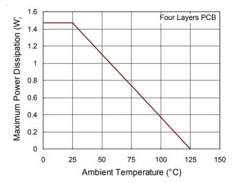
Figure 2. Derating Curves for RT8058 Package
