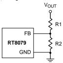
Figure 1. Setting the Output Voltage
