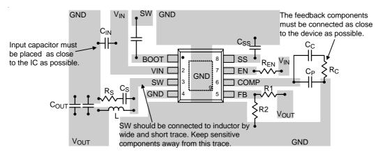
Figure 8. PCB Layout Guide
