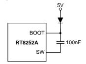
Figure 2. External Bootstrap Diode
