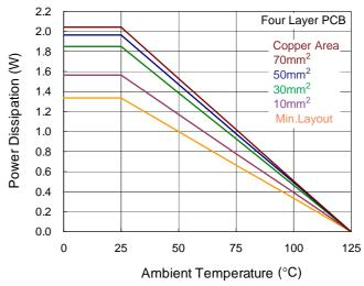
Figure 7. Derating Curves for RT8252A Package
