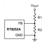
Figure 1. Output Voltage Setting
