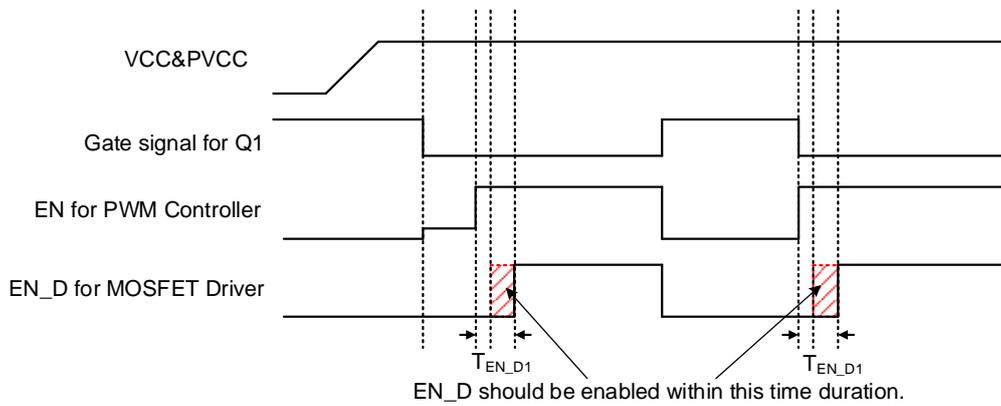
Figure 5. EN Sequence Control Diagram when Middle Drive Function is Enabled
