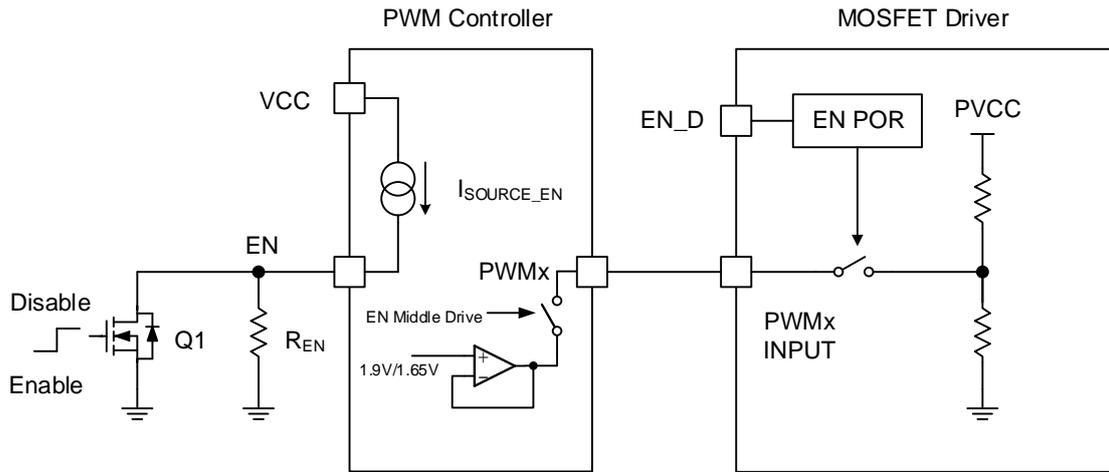
Figure 4. Enable Sequence Control Circuit
