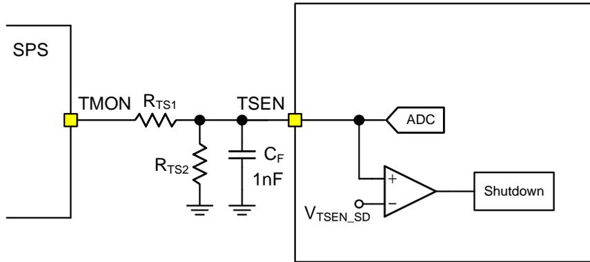
Figure 17. TSEN Pin Application Circuit in SPS Mode
