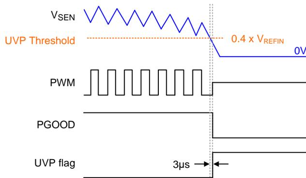
Figure 14. Typical UVP Protection Mechanism
