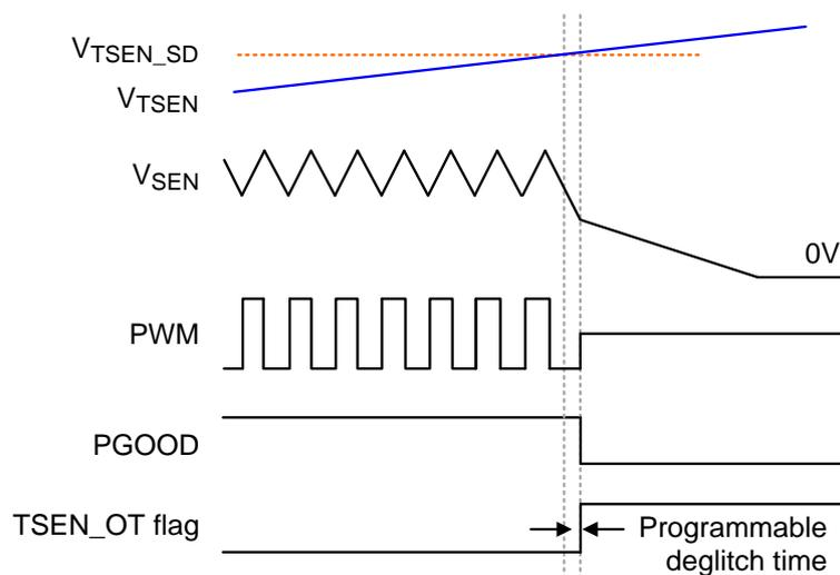
Figure 18. TSEN OTP Protection Mechanism with NTC or PTC
