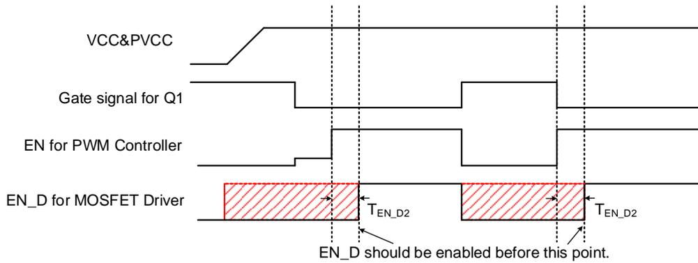
Figure 6. EN Sequence Control Diagram when Middle Drive Function is Disabled
