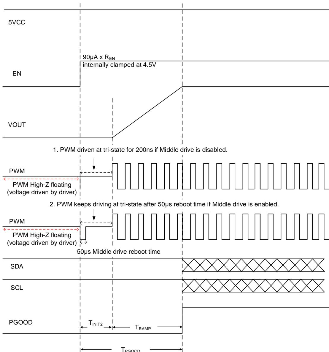
Figure 8. Power-On Sequence of RT8848C by EN re-toggle After First Power-On
