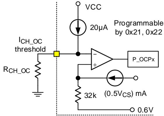
Figure 21. Per-Phase OCP Protection Circuit
