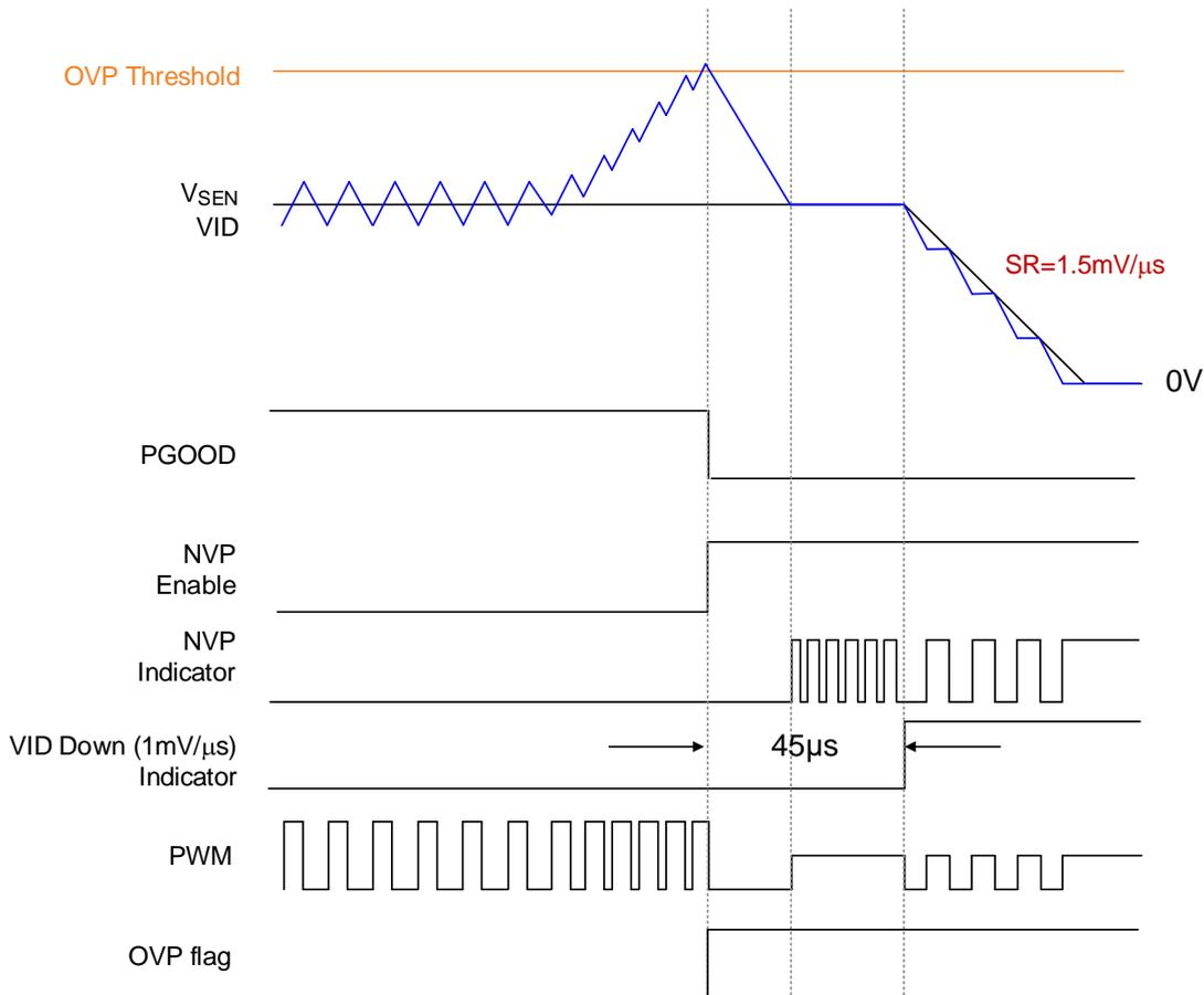
Figure 13. Output Overvoltage Protection Mechanism
