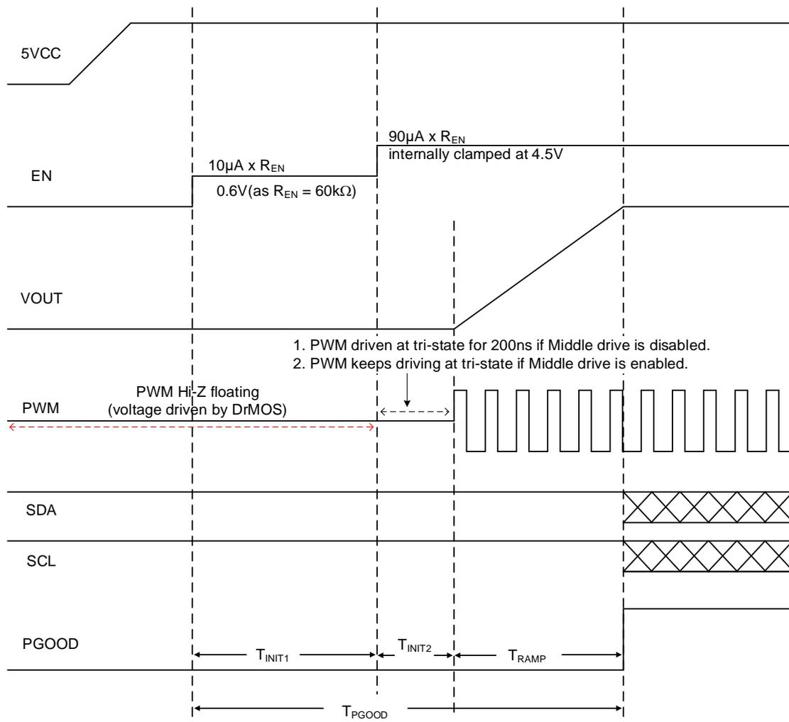
Figure 7. Power-On Sequence of RT8848C at First Power-On
