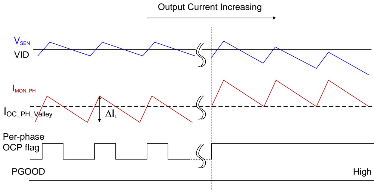
Figure 22. Per-Phase OCP Protection Mechanism
