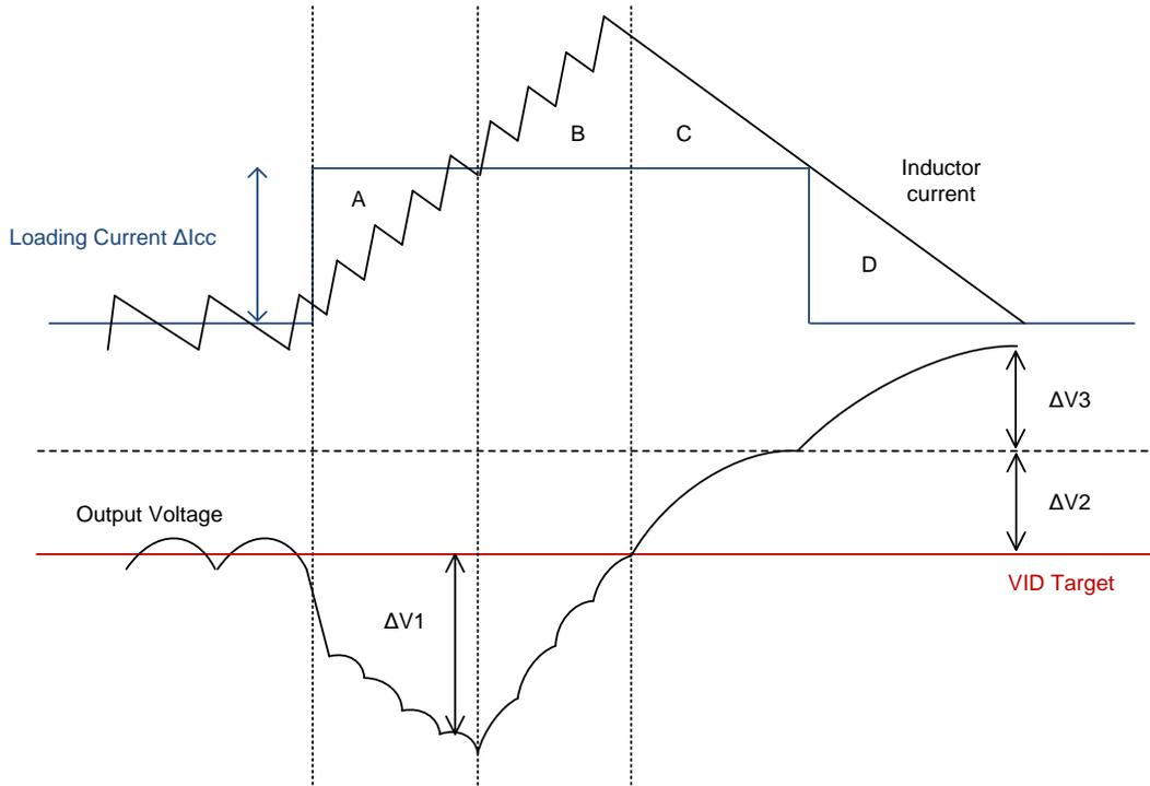
Figure 11. Zero Loadline without AC-droop Control
