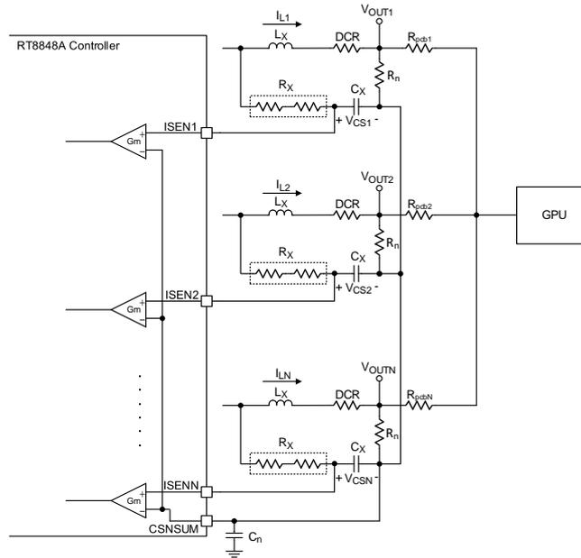
Figure 36. DCR Current Sensing with Common N Structure
