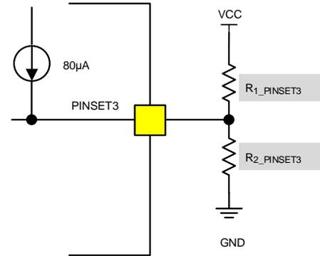
Figure 25. PINSET3 Pin Setting Circuit
