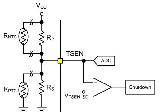
Figure 16. TSEN Pin Application Circuit in DCR Mode
