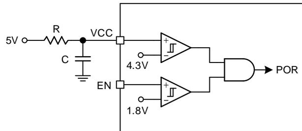
Figure 3. Circuit of Power Ready Detection
