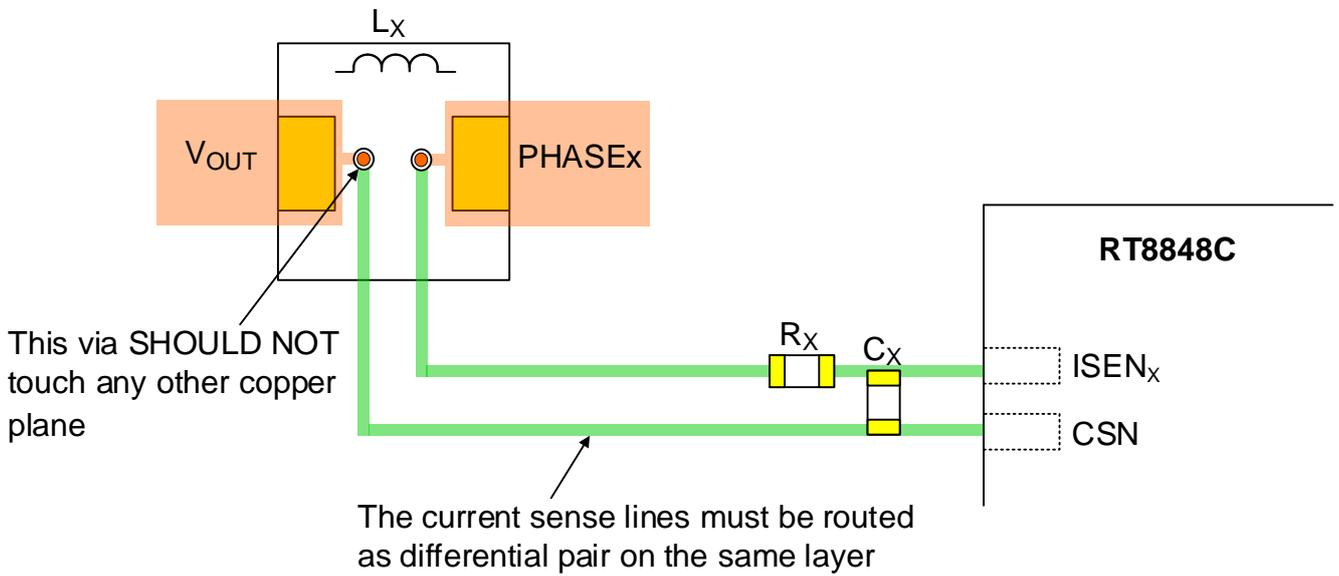
Figure 30. PCB Layout of DCR Current Sensing
