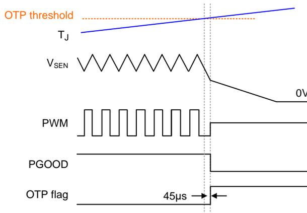
Figure 15. Typical OTP Protection Mechanism
