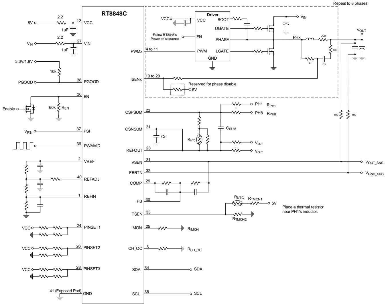
Figure 2. Typical Application Circuit for RT8848C with DCR Current Sense Configuration
