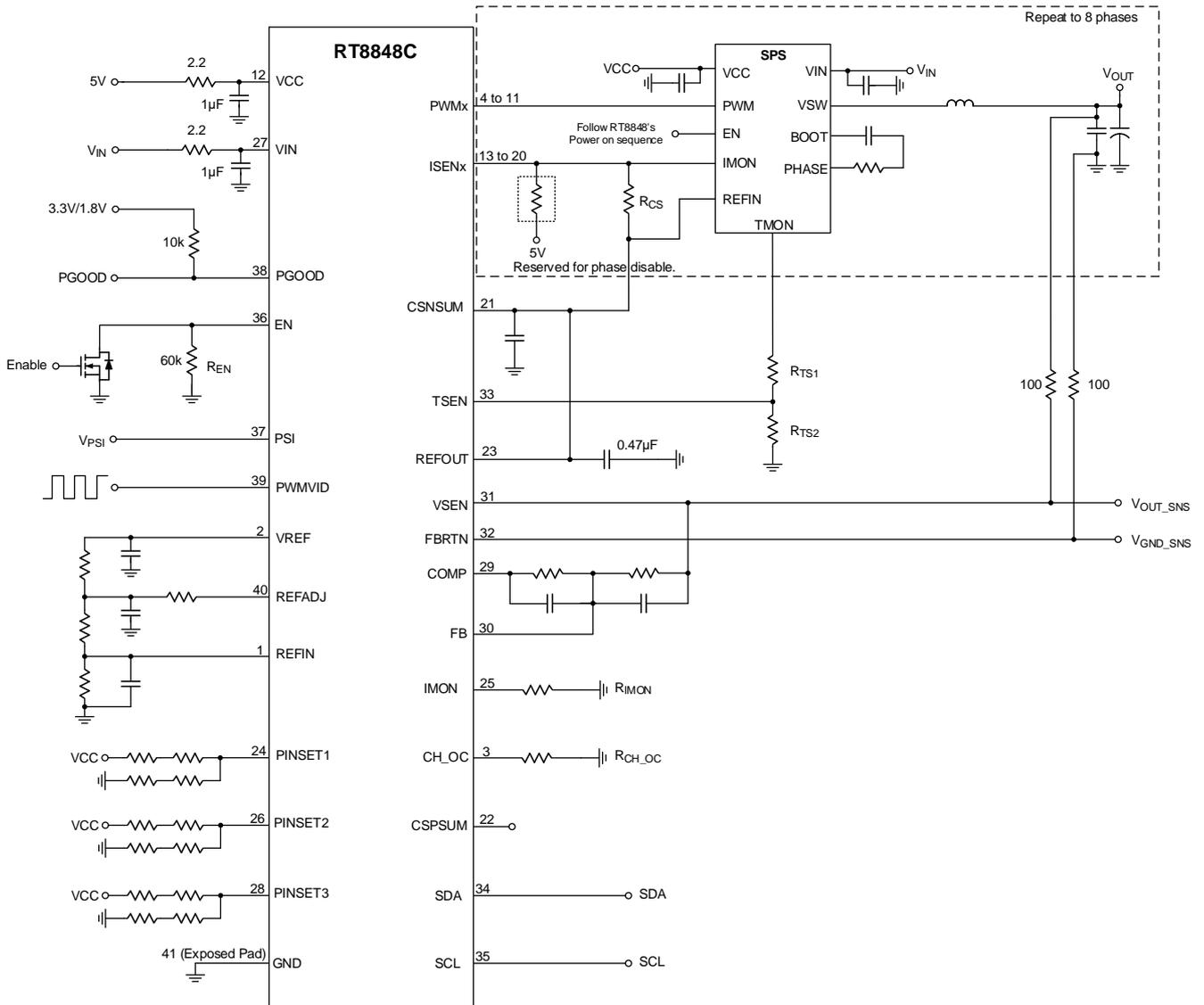
Figure 1. Typical Application Circuit for RT8848C with SPS's IMON Configuration
