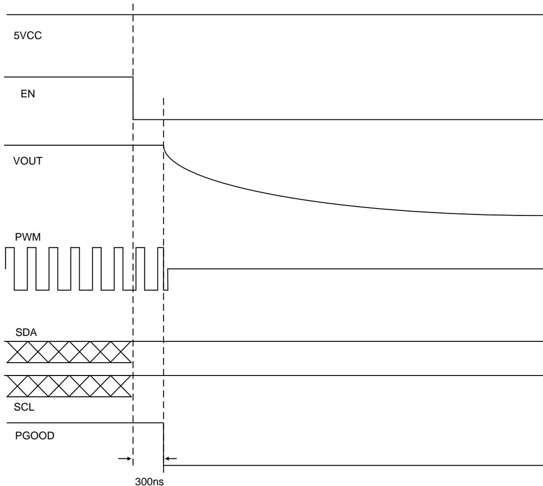
Figure 9. Power-Off Sequence of RT8848C by EN
