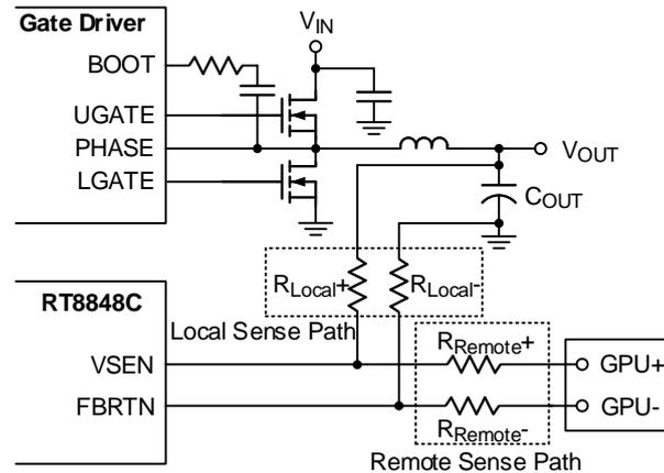
Figure 28. Output Voltage Sensing
