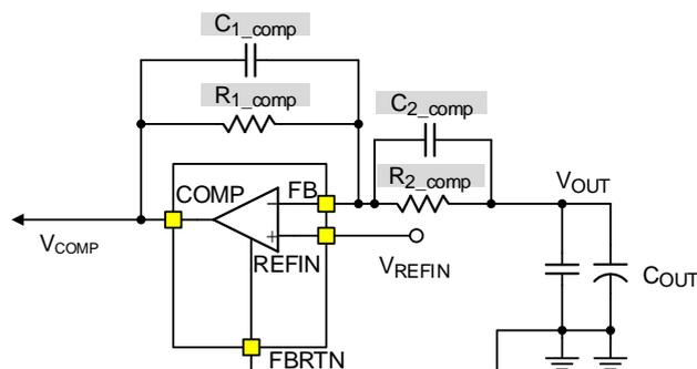
Figure 34. Type I Compensator
