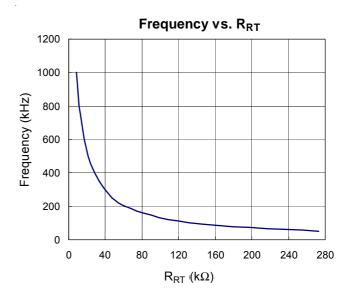
Figure 2. R<sub>RT</sub> vs Phase Switching Frequency
