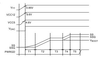
Figure 5. Soft Start Waveforms
