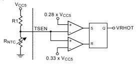
Figure 13. Thermal Monitoring
