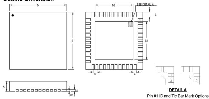
Note: The configuration of the Pin #1 identifier is optional, but must be located within the zone indicated.
