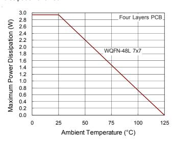
Figure 19. Derating Curves for RT8862 Packages
