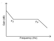
Figure 16. Bode Plot of Type-II Compensation
