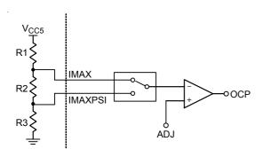
Figure 11. Over Current Protection
