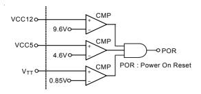
Figure 1. Circuit for Power Ready Detection
