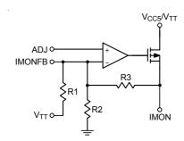
Figure 12. Output Current Monitoring
