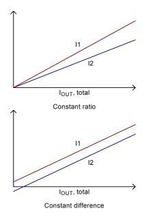
Figure 10. Phase Current vs. Total Current
