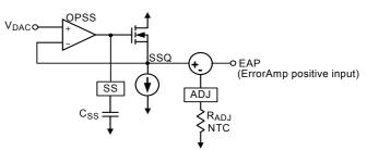
Figure 4. Circuit for Soft Start and Dynamic VID
