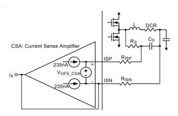
Figure 8. Circuit for Phase Current Sensing
