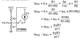
Figure 14. V<sub>PS1</sub> and V<sub>PS2</sub> Setting and Equations
