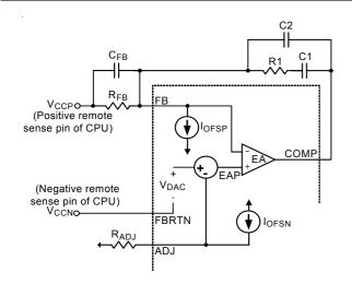
Figure 6. Circuit for V<sub>OUT</sub> Differential Sensing and No Load Offset
