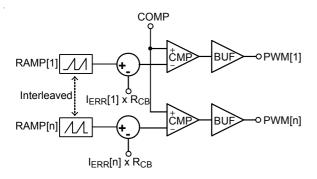
Figure 9. Circuit for Phase Current Balance
