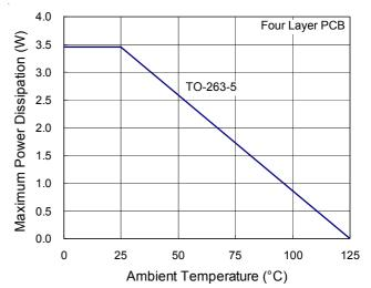
Figure 3. Derating Curves for RT9033 Packages
