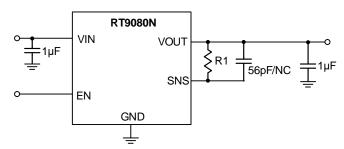
Figure 5. Fine Adjustable Output Voltage Application Circuit
