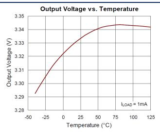
Figure 4. Temperature Coefficient of Adjustable Output Voltage
