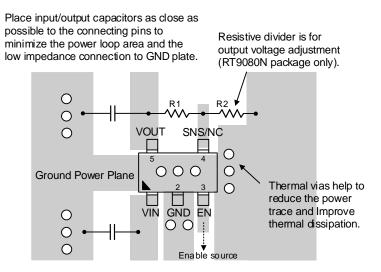
Figure 8. PCB Layout Guide for TSOT-23-5 Package
