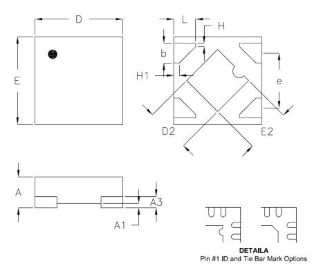
Note: The configuration of the Pin #1 identifier is optional, but must be located within the zone indicated.
