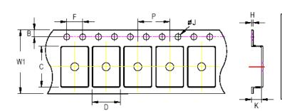
C, D, and K are determined by component size. The clearance between the components and the cavity is as follows:
