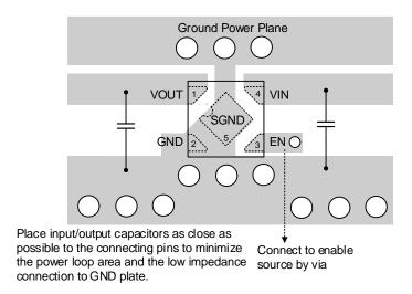
Figure 7. PCB Layout Guide for ZQFN-4L 1x1 Package
