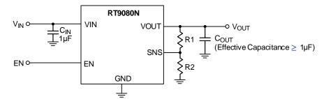
Figure 3. Adjustable Output Voltage Application Circuit
