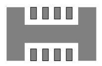
Figure 10 (d). Copper Area =  $50 \text{ mm}^2$ ,  $\theta_{\text{JA}} = 51^{\circ} \text{C/W}$
