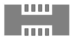
Figure 10 (e). Copper Area =  $70 \text{ mm}^2$ ,  $\theta_{\text{JA}} = 49^{\circ}\text{C/W}$
