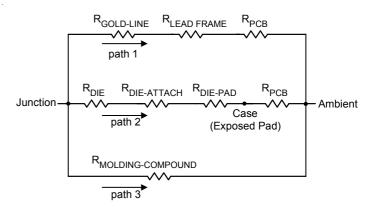
Figure 7. Thermal Resistance Equivalent Circuit
