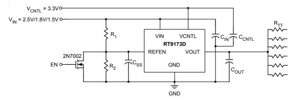
$R_1 = R_2 = 100 k\Omega$ ,  $R_{TT} = 50 \Omega / 33 \Omega / 25 \Omega$
