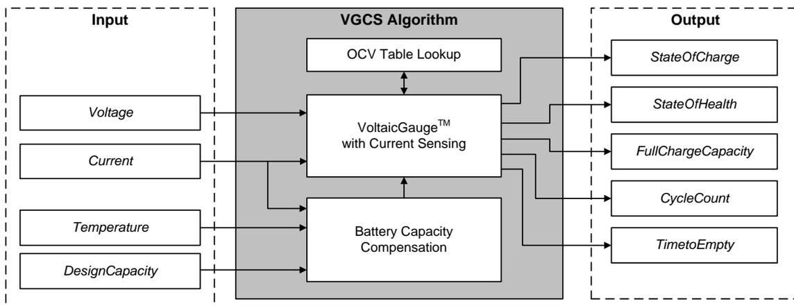
The RT9422 got battery voltage information then using OCV table and iterate calculation with current correction to calculate delta SOC, then using design capacity and battery capacity as a reference to optimize result and output final SOC result. VGCS also support high C-RATE charging technology.
