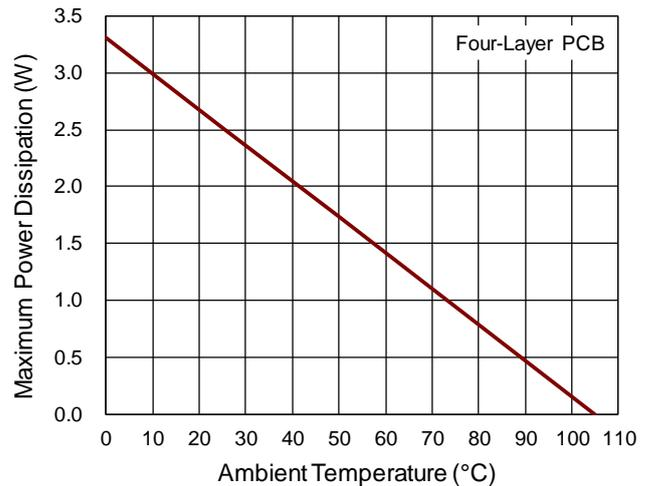
Figure 10. Derating Curve of Maximum Power Dissipation
