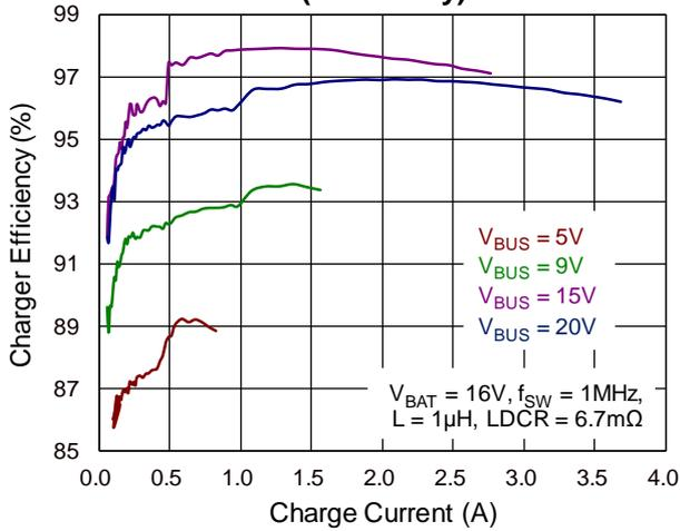
**Charger Efficiency vs. Charge Current
