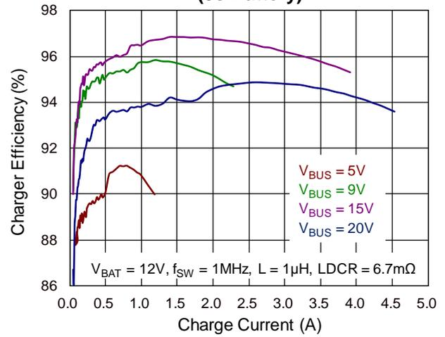
**Charger Efficiency vs. Charge Current
