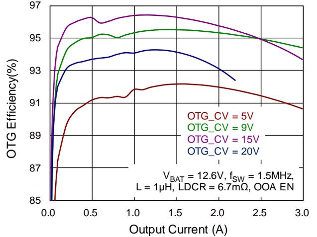
OTG Efficiency vs. Output Current
