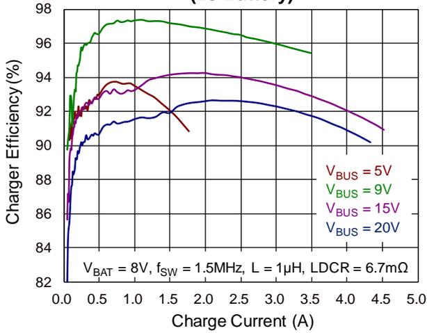
**Charger Efficiency vs. Charge Current
