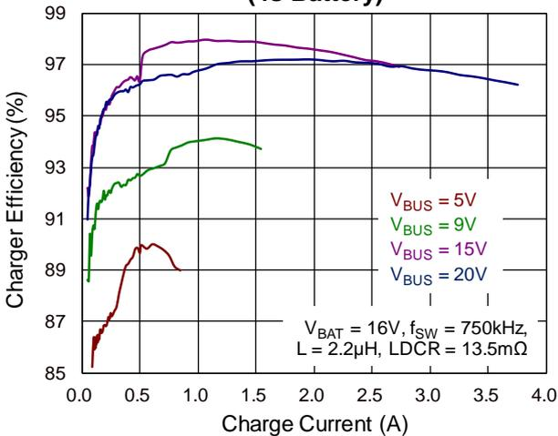
**Charger Efficiency vs. Charge Current
