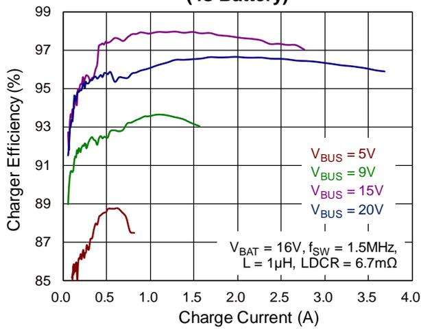
**Charger Efficiency vs. Charge Current
