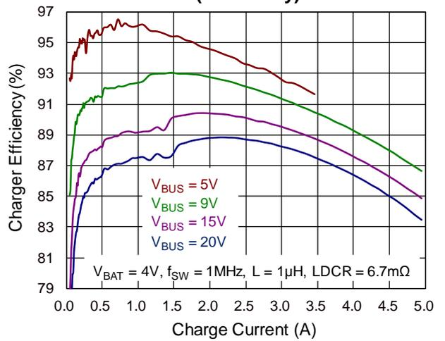
**Charger Efficiency vs. Charge Current
