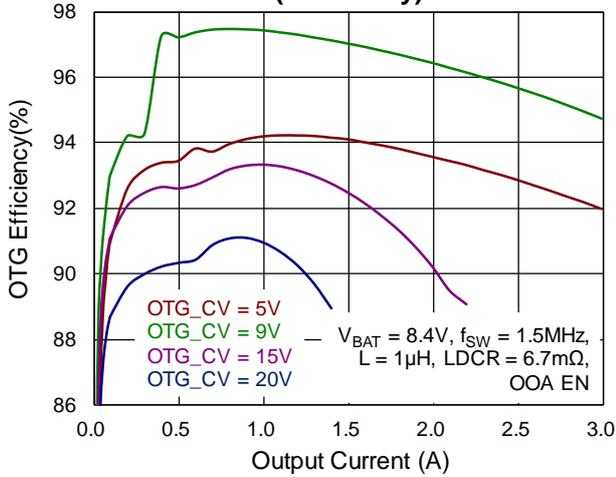
OTG Efficiency vs. Output Current
