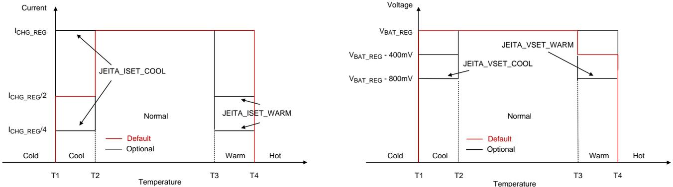
Figure 4. JEITA Protection for Charging Current and Voltage
