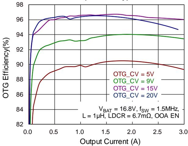
OTG Efficiency vs. Output Current
