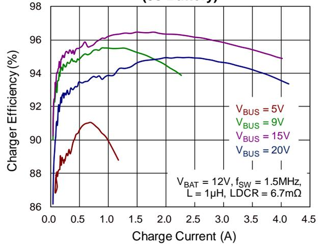
**Charger Efficiency vs. Charge Current
