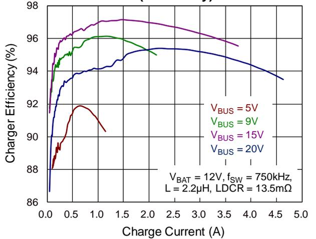
**Charger Efficiency vs. Charge Current
