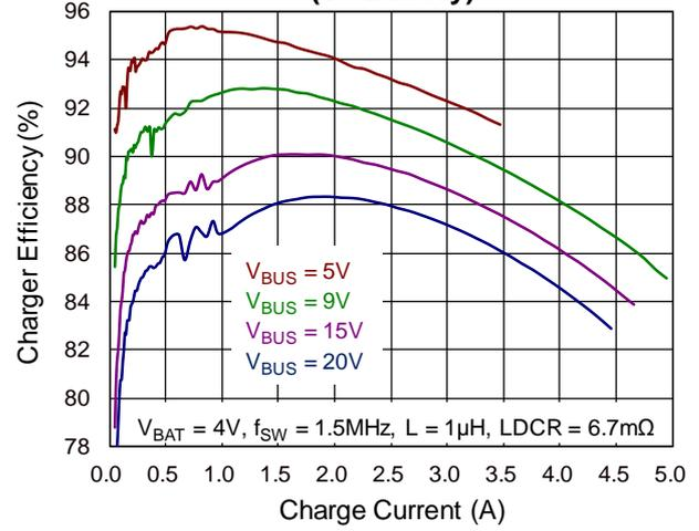
**Charger Efficiency vs. Charge Current
