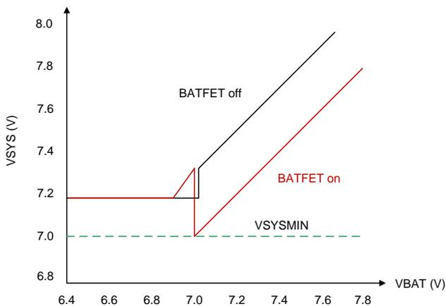
Figure 2. VSYS vs. VBAT for 2s Battery
