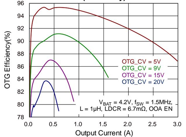
OTG Efficiency vs. Output Current
