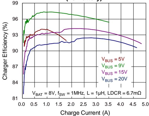
**Charger Efficiency vs. Charge Current
