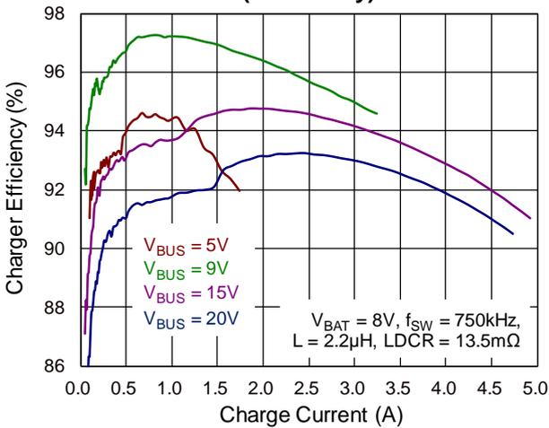
**Charger Efficiency vs. Charge Current
