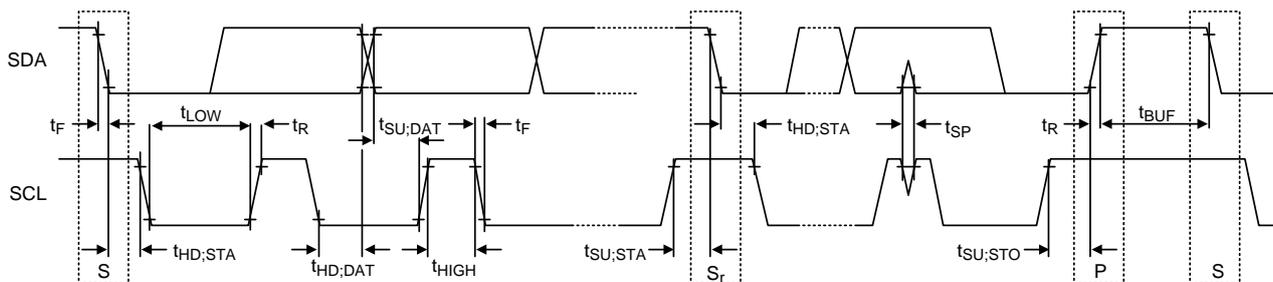
Figure 9. I<sup>2</sup>C Waveform Information
