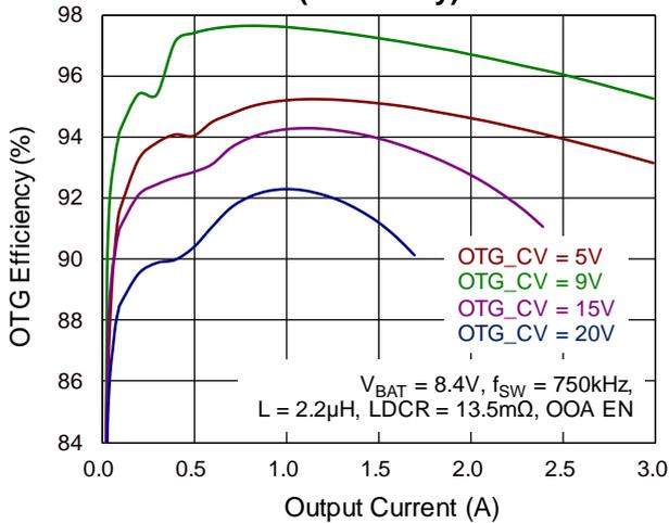
OTG Efficiency vs. Output Current
