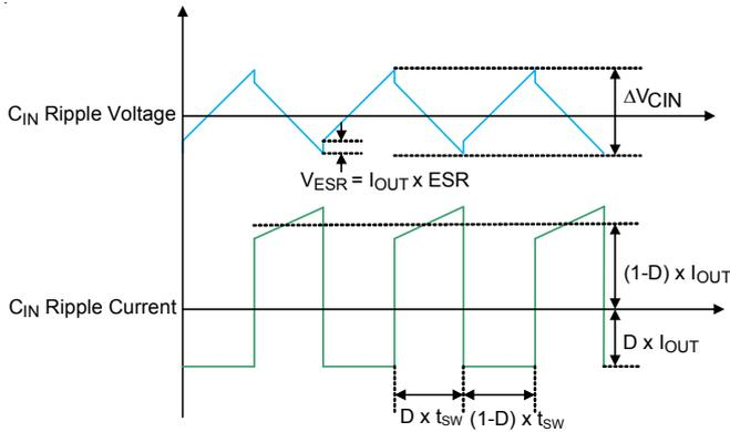
Figure 4.  $C_{IN}$  Ripple Voltage and Ripple Current
