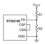
Figure 7. Output Voltage Setting
