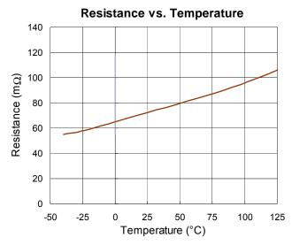
Figure 18. RTQ2105 R<sub>DS(ON)</sub> vs. Temperature
