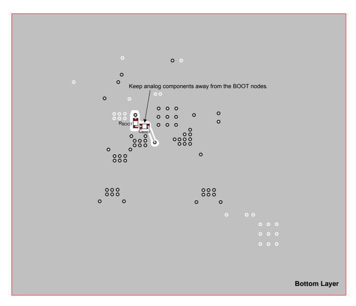
Figure 22. Layout Guide (Bottom Layer)
