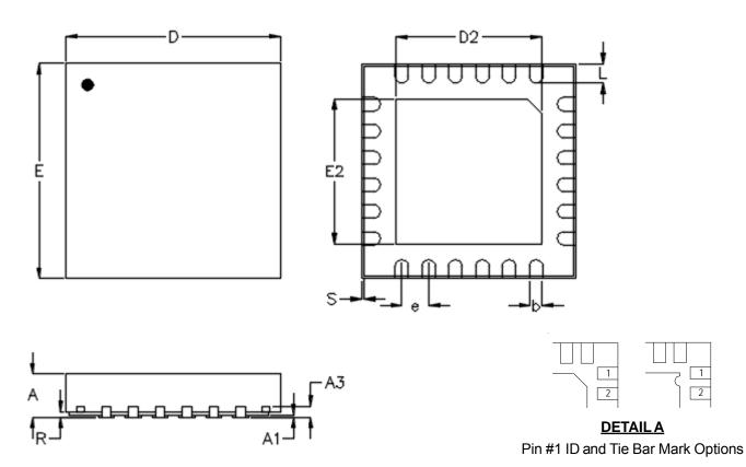
Note: The configuration of the Pin#1 identifier is optional, but must be located within the zone indicated.
