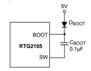
Figure 10. External Bootstrap Diode
