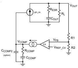
Figure 9. Simplified Equivalent Circuit of Buck with **PCMC**
