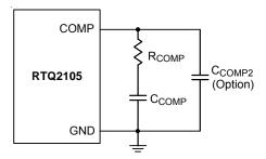
Figure 8. External Compensation Components
