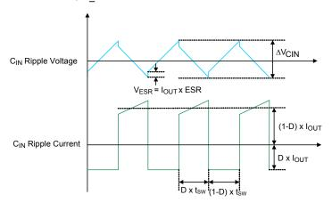
Figure 6. C<sub>IN</sub> Ripple Voltage and Ripple Current
