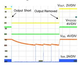
Figure 4. Short Circuit Protection and Recovery
