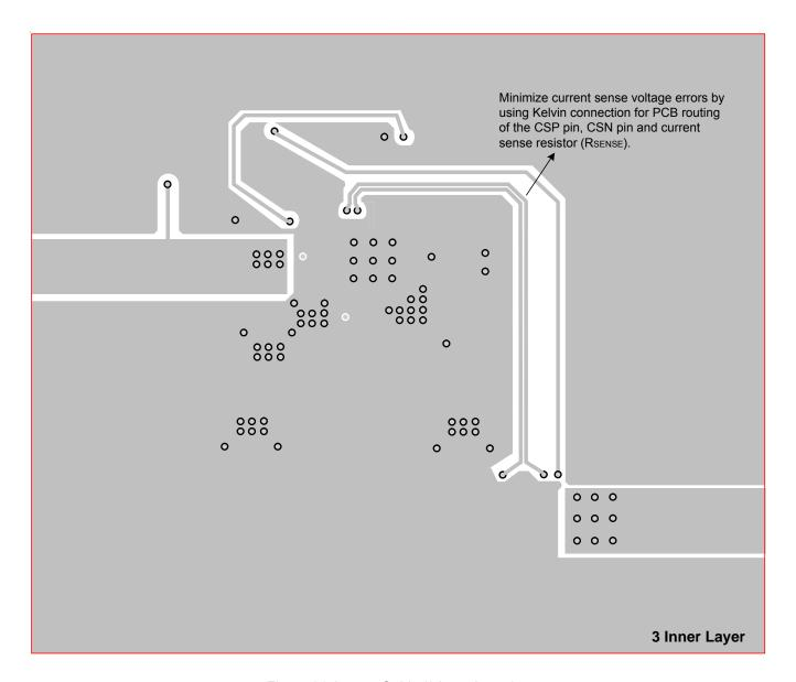
Figure 21. Layout Guide (3 Inner Layer)
