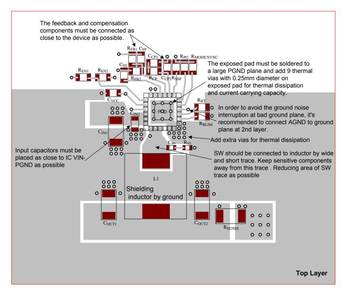
Figure 19. Layout Guide (Top Layer)
