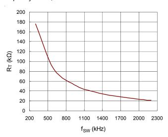
Figure 5. Switching Frequency vs. R<sub>T</sub>
