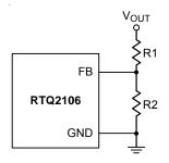
Figure 5. Output Voltage Setting
