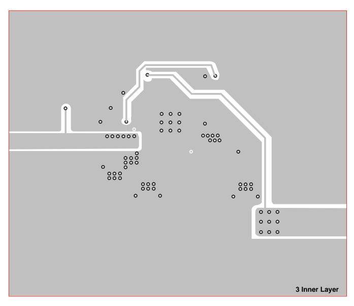
Figure 18. Layout Guide (3 Inner Layer)
