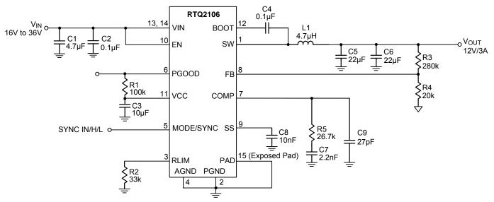
L1 = Cyntec-VCHA075D-4R7MS6 C5/C6 = GCM32EC71E226KE36L C1 = GRM31CR71H475KA12L
