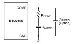
Figure 6. External Compensation Components
