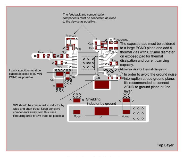
Figure 16. Layout Guide (Top Layer)
