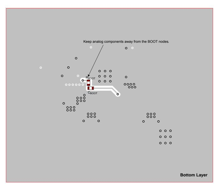
Figure 19. Layout Guide (Bottom Layer)
