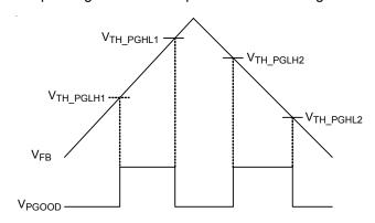
Figure 2. The Logic of PGOOD
