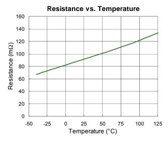
Figure 15. RTQ2106 R<sub>DS(ON)</sub> vs. Temperature
