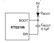
Figure 8. External Bootstrap Diode
