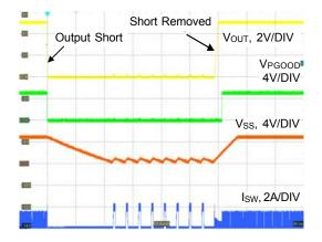
Figure 3. Short Circuit Protection and Recovery
