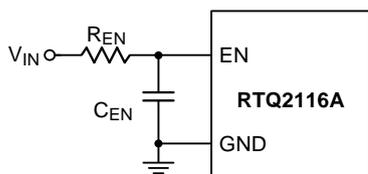
Figure 14. Enable Timing Control
