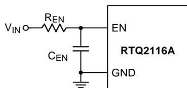
Figure 14. Enable Timing Control
