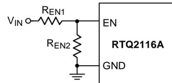
Figure 16. Resistive Divider for Under-Voltage Lockout Threshold Setting
