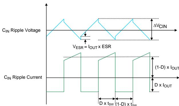
Figure 6. C<sub>IN</sub> Ripple Voltage and Ripple Current
