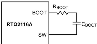
Figure 12. External Bootstrap Resistor at the BOOT Pin
