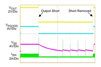
Figure 4. Short Circuit Protection and Recovery
