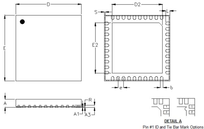
Note : The configuration of the Pin #1 identifier is optional,
