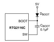
Figure 15. External Bootstrap Diode
