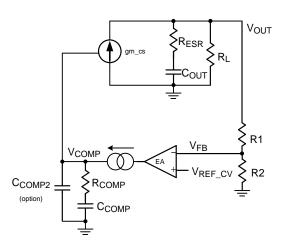
Figure 14. Simplified Equivalent Circuit of Buck with PCMC
