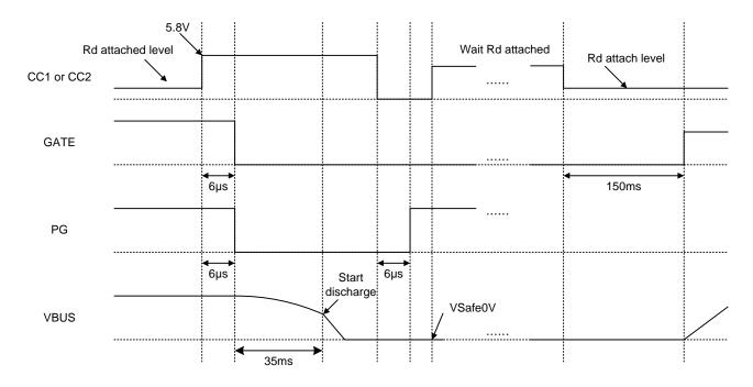
Figure 9. CC Over-Voltage Protection Sequence
