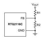
Figure 12. Output Voltage Setting
