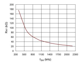
Figure 10. Switching Frequency vs. R<sub>RT</sub> Resistor
