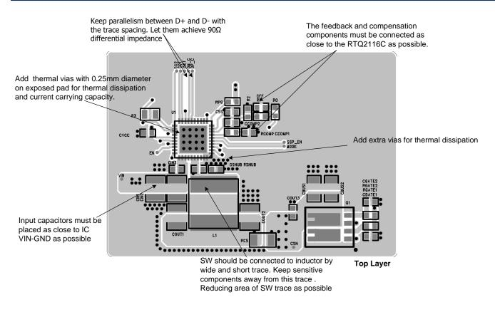
Figure 24. Layout Guide (Top Layer)
