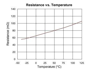
Figure 23. Resistance Variation Curve at Different Temperature
