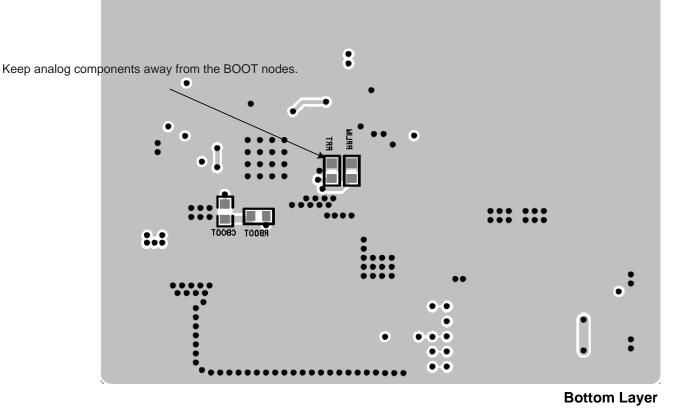
Figure 27. Layout Guide (Bottom Layer)
