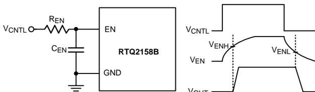
Figure 10. Enable Timing Control
