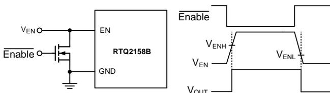
Figure 11. Logic Control for the EN Pin
