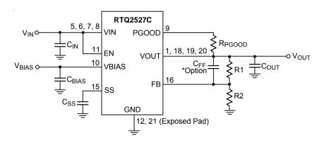
\*: The feedforward capacitor is optional for the transient response and circuit stability improvement.
