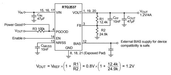
Figure 1. Configuration Circuit for V<sub>OUT</sub> Adjusted by a Resistive Divider
