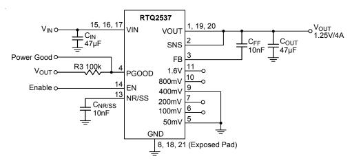
$V_{OUT} = V_{REF} + 50mV + 400mV = 0.8V + 50mV + 400mV = 1.25V$
