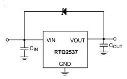
Figure 7. Application Circuit for Reverse Current Protection
