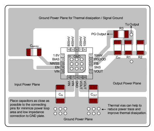
Figure 9. PCB Layout Guide
