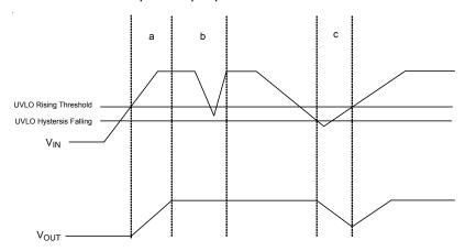
Figure 5. Under-Voltage Lockout Trigging Conditions and Output Variation
