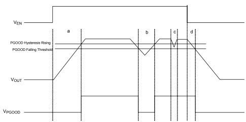
Figure 6. PGOOD Trigger Scenario with Different Operating Status
