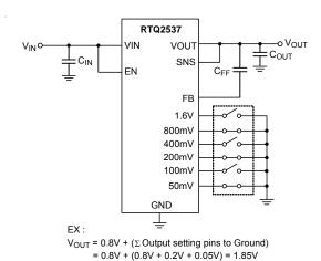
Figure 4. Output Setting without External Resistors
