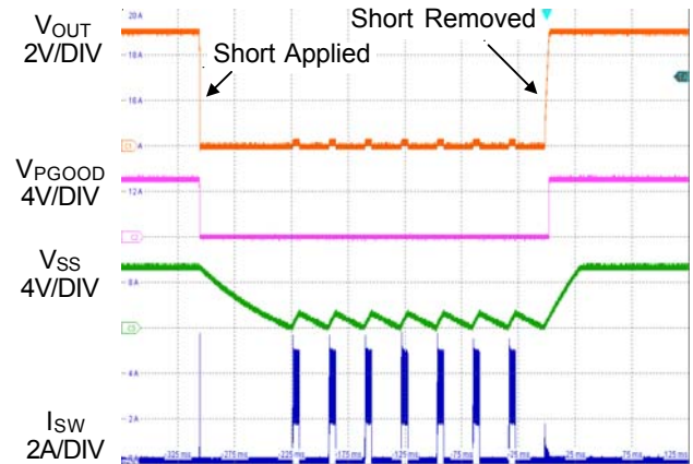
Figure 3. Short-Circuit Protection and Recovery
