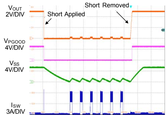
Figure 3. Short-Circuit Protection and Recovery
