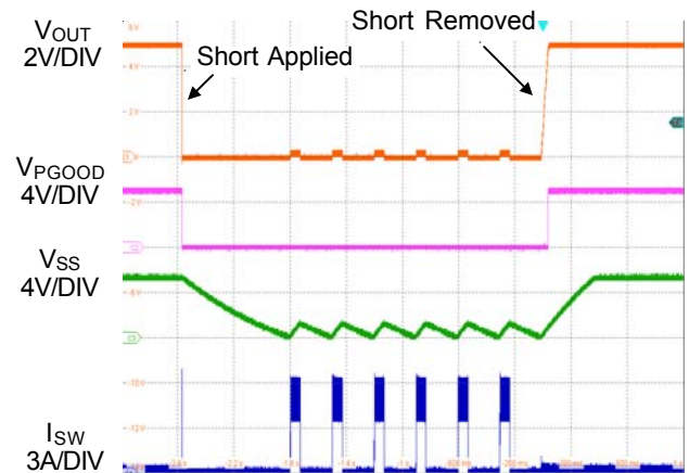
Figure 3. Short-Circuit Protection and Recovery
