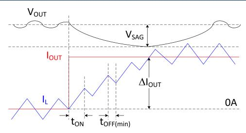
Figure 16. Output Voltage Drop (VSAG) Estimation as Output Load Current Step Up
