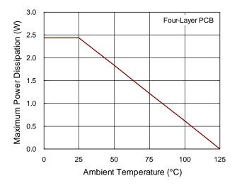
Figure 20. Derating Curve of Maximum Power Dissipation
