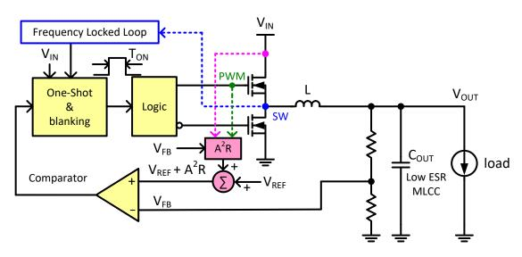
Figure 10. A<sup>2</sup>RCOT Control Mechanism
