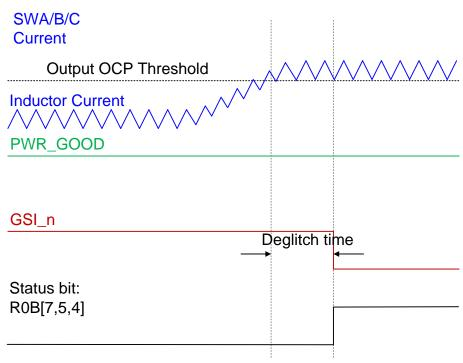
Figure 9. Output Current Limiter Protection
