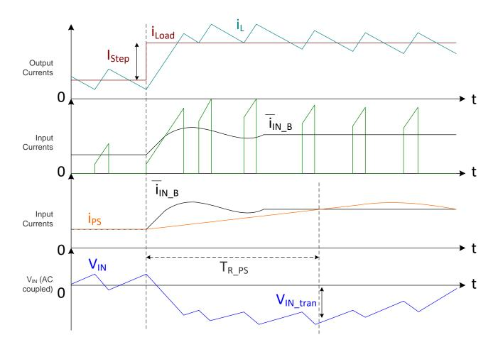
Figure 18. VIN Transient Current Diagram
