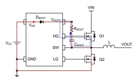
Figure 19. Bootstrap Power Supply Circuit
