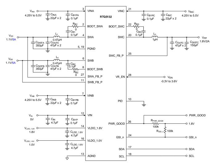
Figure 14. Typical Application Circuit when SWA and SWB are separated for 2-Outputs.
