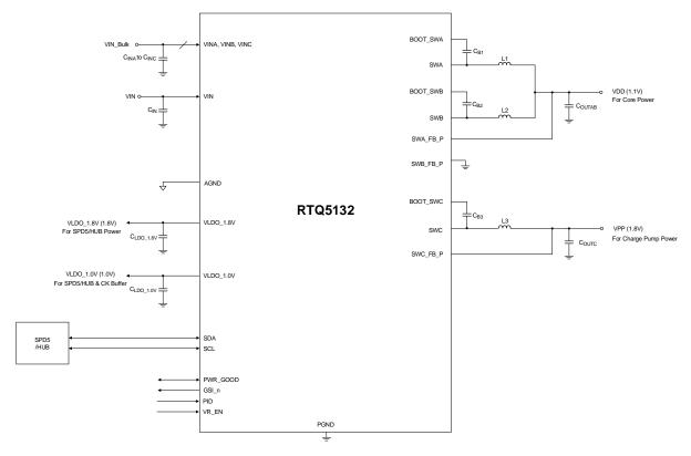
Figure 1. SWA and SWB are combined as Dual-Phase Mode
