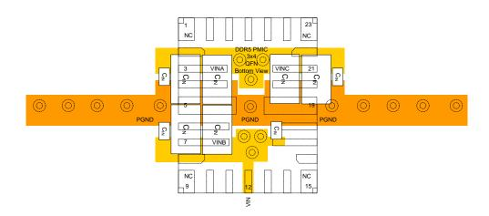
Figure 22. RTQ5132 Layout Guide (Bottom Layer)
