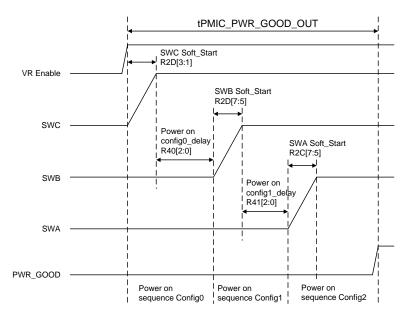
Figure 7. RTQ5132 Rails Power On Timing
