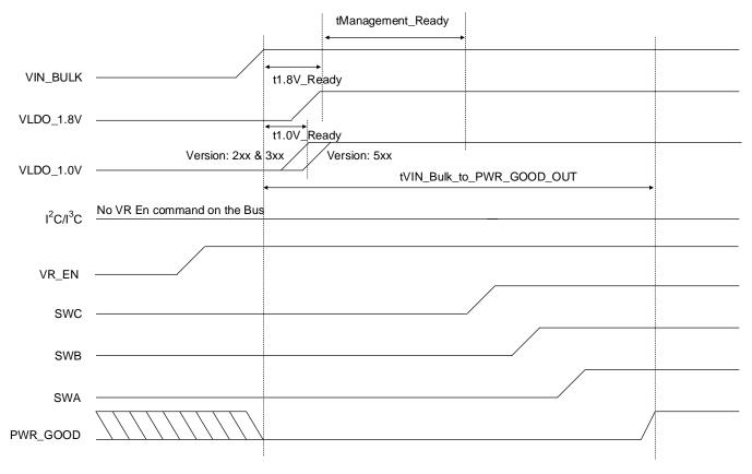
Figure 4. Power Up Sequence; VR\_EN pin High before VIN\_Bulk Ramp; No Bus Command
