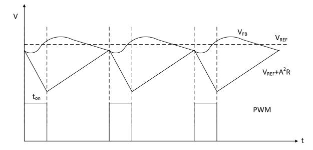
Figure 11. A<sup>2</sup>RCOT PWM Control Diagram
