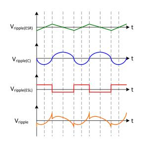
Figure 15. Output Ripple Decomposition
