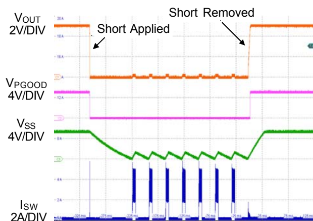
Figure 3. Short-Circuit Protection and Recovery
