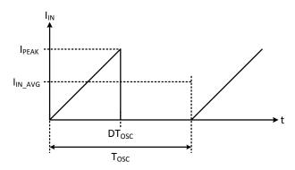
need to define the point at which the inductor current ripple touches zero, and as the power switch SW is immediately reactivated, the current ramps up again. Figure 10 portrays the input current activity of the buckboost converter.
