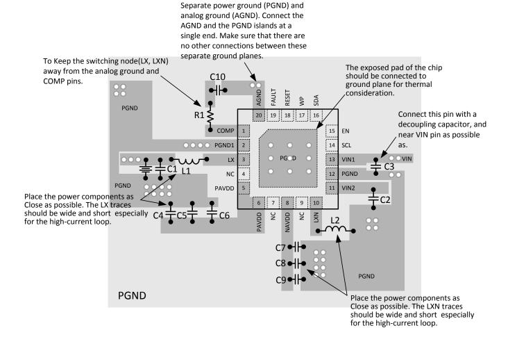
Figure 14. PCB Layout Guide
