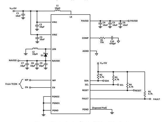
Figure 2. The Application Circuit of VIN > 4V Application
