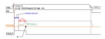
Figure 6. SCP Mechanism at PAVDD pre-charge when PAVDD with the Abnormal Heavy Load
