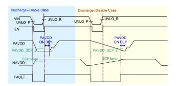
Figure 5. The Power-up Limitation of The Outputs
