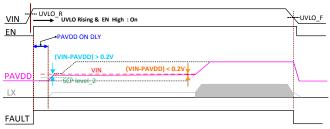
Figure 7. SCP Mechanism when PAVDD between SCP Level and Pre-charge Finish
