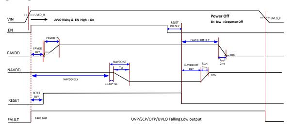
Figure 3. Power Sequence with Sequence Power-Off
