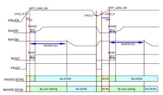
Figure 11. Discharge Function Enable Operation
