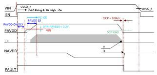
Figure 8. SCP Mechanism during Normal Operating
