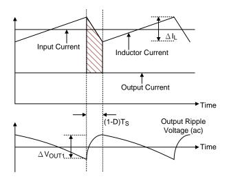
Figure 9. The Output Ripple Voltage without the Contribution of ESR
