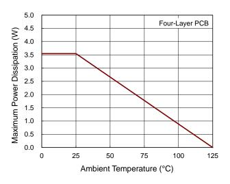
Figure 13. Derating Curve of Maximum Power
