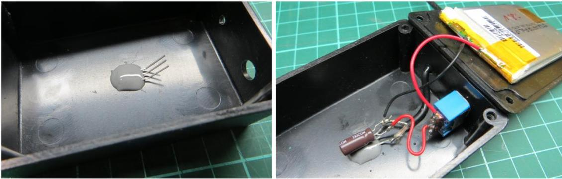
Then the sensor is fixed with non-transparent epoxy glue. Finally the other components are connected.
