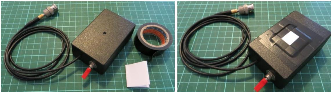
Due to the high light sensitivity of the TSL257, the incoming light to the sensor needs to be attenuated considerably to make it suitable for measuring direct light from LED strings. Several layers of A4 paper can be placed over the hole to achieve sufficient light attenuation. For the test tool, 8 layers of paper were used.
