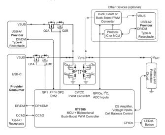
As shown in the diagram,  $Q_A$ ,  $Q_B$ ,  $Q_C$ ,  $Q_D$  switches and L1 inductor are key components for the bi-directional Buck-Boost controller.  $Q_{1A}$  and  $Q_{1B}$  switches are the external output blocking MOSFETs between the output of the PWM converter and the USB Type-C VBUS terminal.
