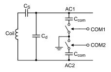
Figure 10. Capacitive Load Modulation
