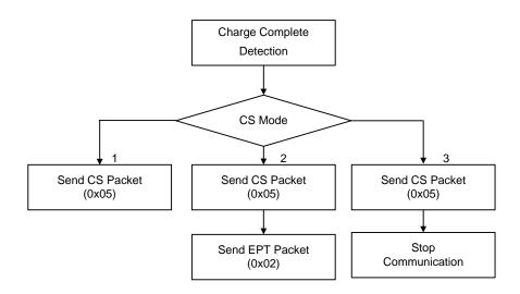
Figure 15. Operation Modes of Charge Complete Detection
