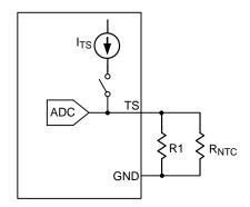
Figure 5. NTC Circuit for Device Temperature
