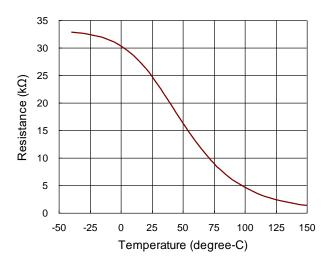
Figure 8. Equivalent Resistance for Temperature
