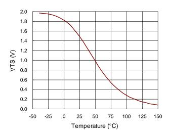
Figure 9. Thermal Sensing Voltage
