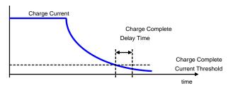
Figure 14. Battery Charge Complete Detection
