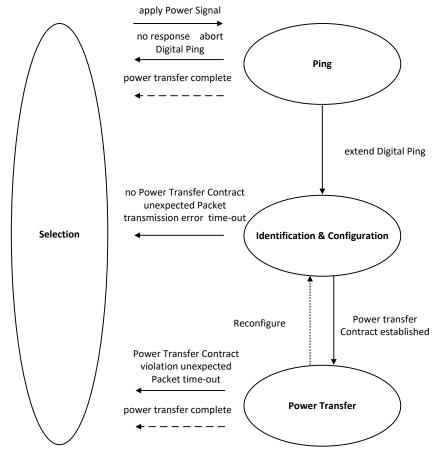
Figure 2. WPC V1.2 Low Power Transfer Phases
