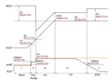
Figure 13. Battery Charge Behavior
