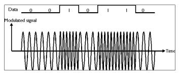
Figure 11. FSK Modulation Power Signal
