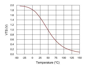
Figure 9. Thermal Sensing Voltage
