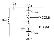
Figure 10. Capacitive Load Modulation
