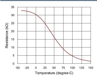
Figure 8. Equivalent Resistance for Temperature Sensing
