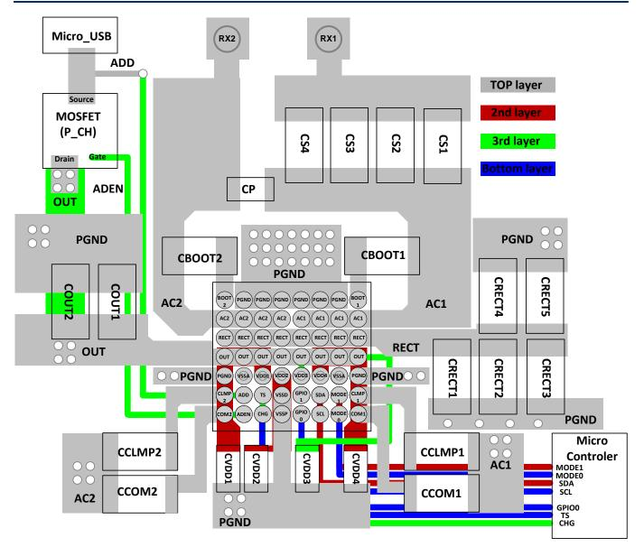
Figure 17. PCB Layout Guide
