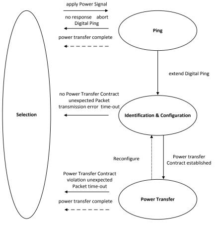
Figure 2. WPC V1.2.4 Low Power Transfer Phases
