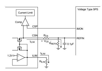
Figure 6. Current Limit Setting for Voltage Type SPS
