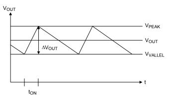
Figure 9. Output Voltage Waveform
