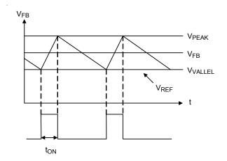
Figure 1. Constant On-Time PWM Control
