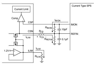
Figure 7. Current Limit Setting for Current Type SPS
