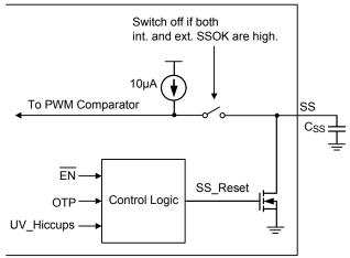
Figure 3. Soft-Start Control Block.
