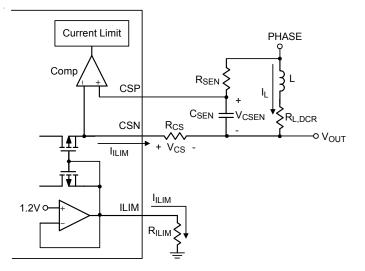
Figure 5. Current Limit Setting for DCR Current Sense
