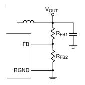
Figure 10. Setting with a Resistive Voltage Divider
