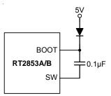
Figure 5. External Bootstrap Diode
