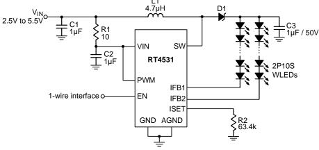
Figure 1. RT4531 1-wire Dimming Typical Application
