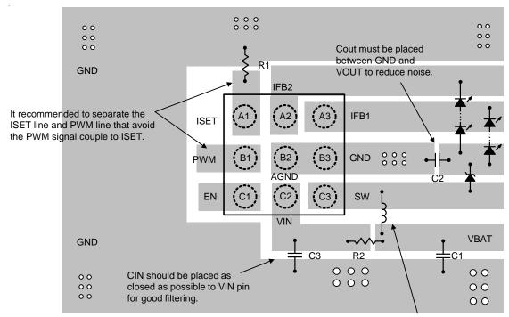
The inductor should be placed as close as possible to the switch pin to minimize the noise coupling into other circuits. SW node copper area should be minimized for reducing EMI.
