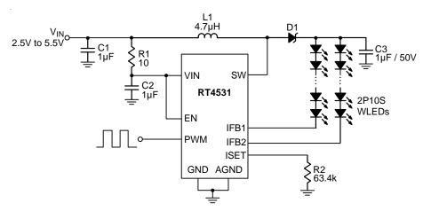
Figure 2. RT4531 PWM Dimming Typical Application
