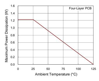
Figure 3. Derating Curve of Maximum Power Dissipation
