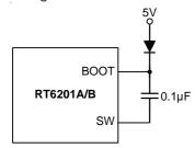
Figure 5. External Bootstrap Diode
