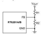
Figure 4. Output Voltage Setting
