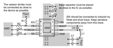
Figure 7. PCB Layout Guide
