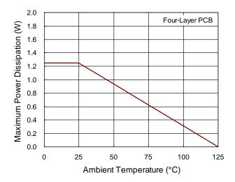
Figure 7. Derating Curve of Maximum Power
