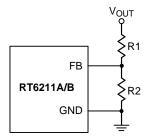
Figure 5. Output Voltage Setting
