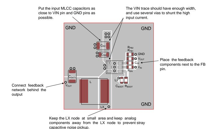
Figure 8. PCB Layout Guide
