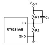
Figure 1. Cff Capacitor Setting
