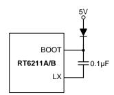
Figure 6. External Bootstrap Diode
