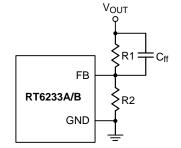
Figure 1. Cff Capacitor Setting
