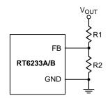
Figure 5. Output Voltage Setting
