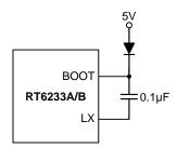
Figure 6. External Bootstrap Diode
