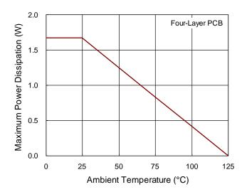
Figure 7. Derating Curve of Maximum Power Dissipation
