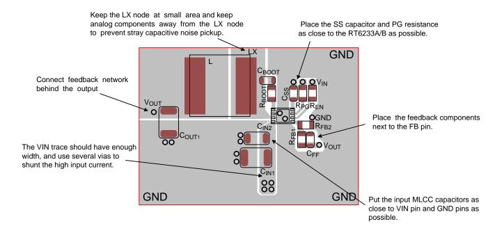
Figure 8. PCB Layout Guide
