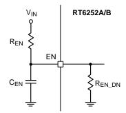
Figure 7. External Timing Control
