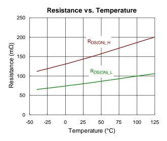
Figure 13. RT6252A/B R<sub>DS(ON)</sub> vs. Temperature
