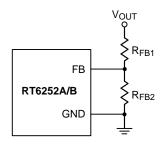
Figure 2. Output Voltage Setting
