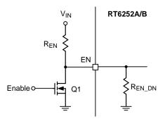
Figure 8. Digital Enable Control Circuit
