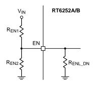
Figure 9. Resistor Divider for Lockout Threshold Setting
