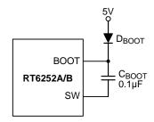
Figure 10. External Bootstrap Diode
