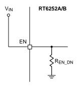
Figure 6. Automatic Start-Up Setting
