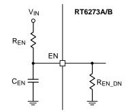
Figure 7. External Timing Control
