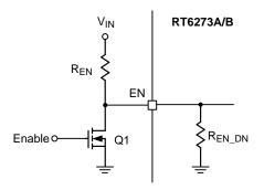
Figure 8. Digital Enable Control Circuit
