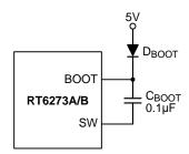
Figure 10. External Bootstrap Diode
