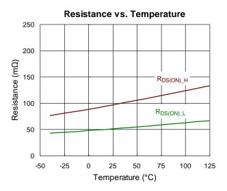
Figure 13. RT6273A/B R<sub>DS(ON)</sub> vs. Temperature
