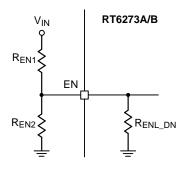
Figure 9. Resistor Divider for Lockout Threshold
