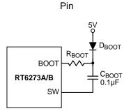
Figure 12. External Bootstrap Diode and Resistor at the BOOT Pin
