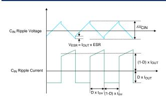
Figure 1.  $C_{\text{IN}}$  Ripple Voltage and Ripple Current In addition, the input capacitor needs to have a very low ESR and must be rated to handle the worst-case RMS input current of :
