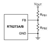
Figure 2. Output Voltage Setting
