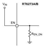
Figure 6. Automatic Start-Up Setting
