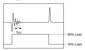
Figure 4. Example of Measuring the Converter BW by **Fast Load Transient**
