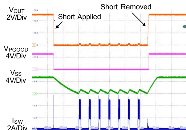
Figure 3. Short Circuit Protection and Recovery
