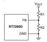
Figure 5. Output Voltage Setting
