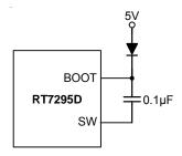
Figure 6. External Bootstrap Diode
