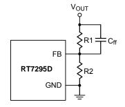
Figure 1. Cff Capacitor Setting
