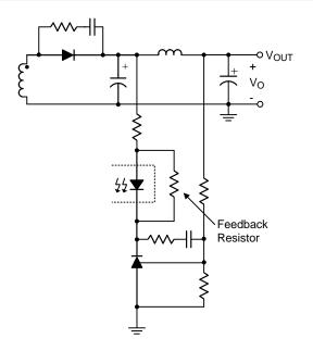
Figure 9. Feedback Resistor
