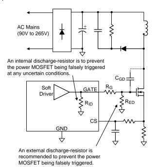
Figure 8. Resistors at the GATE Pin
