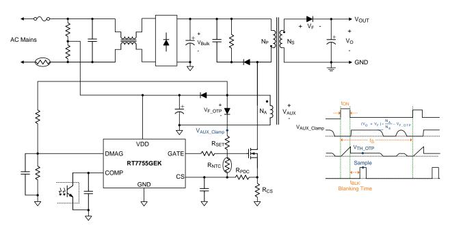
Figure 7. Application Circuit of External Over-Temperature Protection
