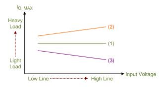
Figure 6. Output Current Limits for Over-Current Protection
