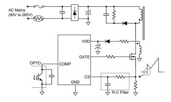
Figure 10. R-C Filter on the CS Pin
