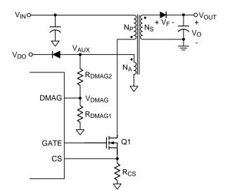
Figure 3. DMAG Pin Resistor
