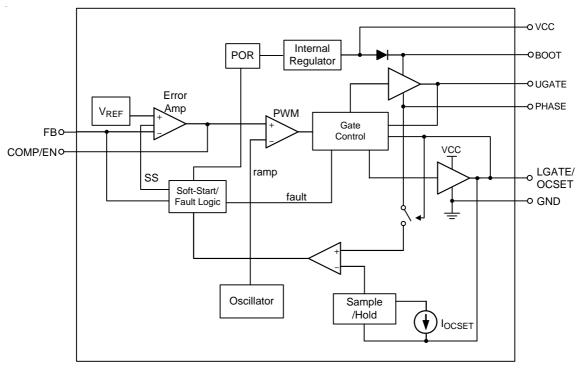
Figuer 1. RT8120A/B Function Block Diagram
