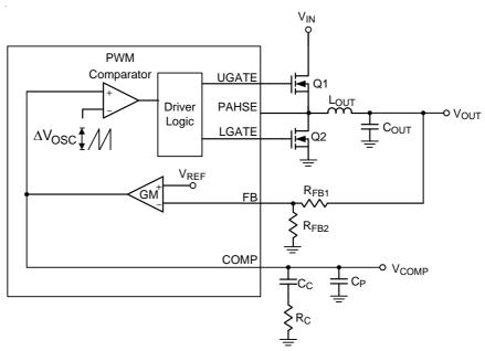
Figure 5. Typical Voltage Mode Buck Converter Control Loop
