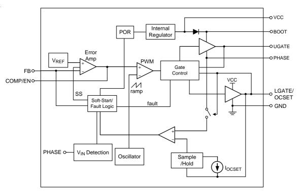
Figuer 2. RT8120C/D Function Block Diagram
