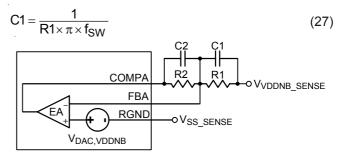
Figure 17. VDDNB Controller: Compensation Circuit
