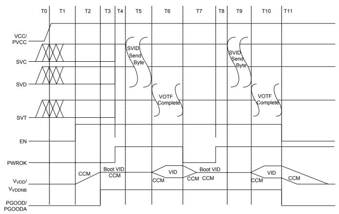
Figure 3. Simplified Sequence Timing Diagram
