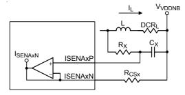
Figure 19. VDDNB Controller: Lossless Inductor Sensing
