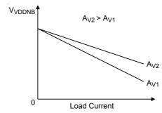
Figure 16. VDDNB Controller: Error Amplifier gain (A<sub>V</sub>) Influence on V<sub>VDDNB</sub> Accuracy
