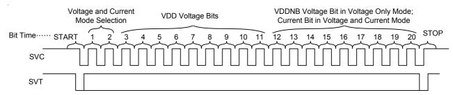
Figure 4. Telemetry Bit Definition
