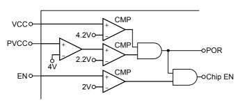
Figure 1. Power Ready (POR) Detection
