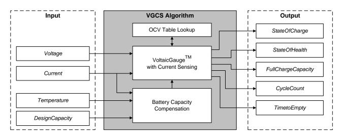
The RT9427 got battery voltage information then using OCV table and iterate calculation with current correction to calculate delta SOC, then using design capacity and battery capacity as a reference to optimize result and output final SOC result.
