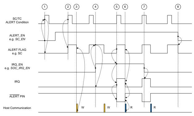
Figure 2. SC/TC ALERT Function Timing Diagram
