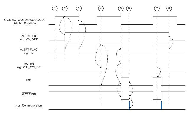
Figure 1. ALERT Function Timing Diagram
