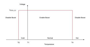
Figure 7. Thermal Protect During Boost Mode
