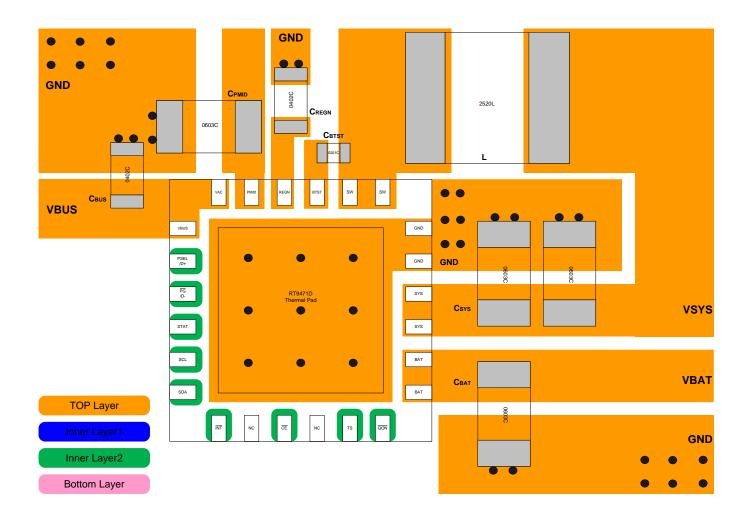
Figure 13. PCB Layout Guide for the RT9471D
