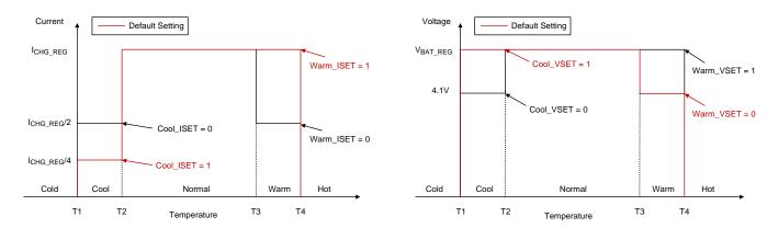
Figure 6. JEITA Protect for Charging Current and Voltage
