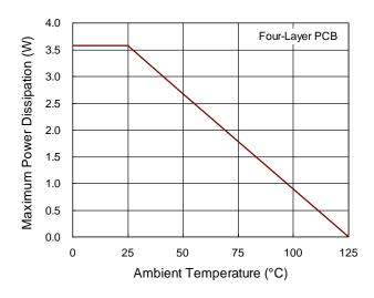
Figure 11. Derating Curve of Maximum Power Dissipation
