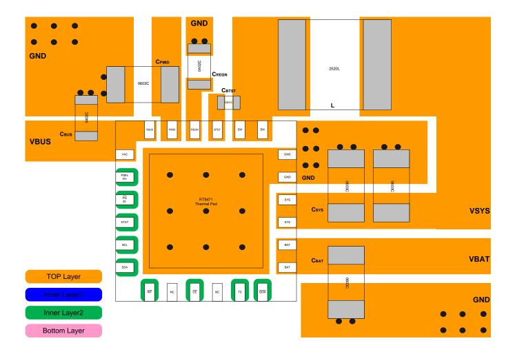
Figure 12. PCB Layout Guide for the RT9471
