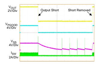
Figure 3. Short Circuit Protection and Recovery
