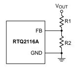
Figure 7. Output Voltage Setting
