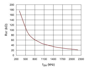
Figure 5. Switching Frequency vs. RRT Resistor
