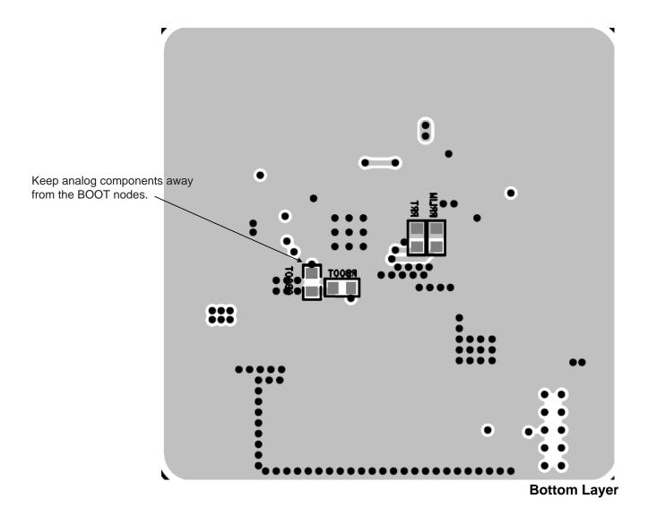
Figure 22. Layout Guide (Bottom Layer)
