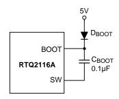
Figure 10. External Bootstrap Diode
