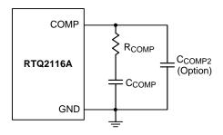
Figure 8. External Compensation Components
