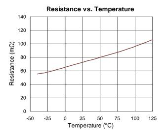
Figure 18. Resistance Variation Curve at Different Temperature
