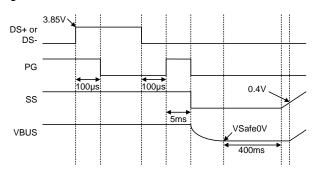
Figure 4. Data Over Voltage Protection Sequence
