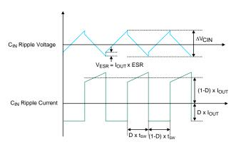
Figure 6. C<sub>IN</sub> Ripple Voltage and Ripple Current
