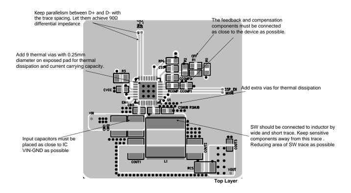
Figure 19. Layout Guide (Top Layer)
