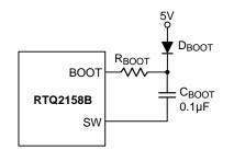
Figure 5. External Bootstrap Diode and Resistor at the BOOT Pin
