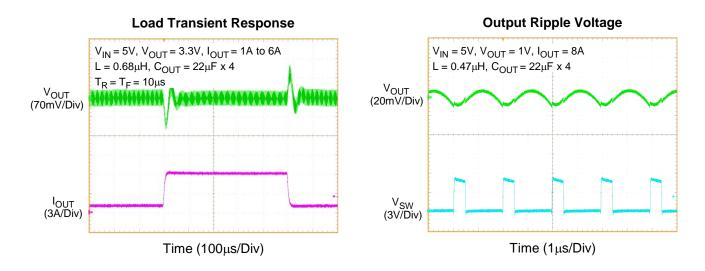
$L = 0.68 \mu H$ ,  $C_{OUT} = 22 \mu F \times 4$  $T_R = T_F = 10 \mu s$
