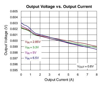
**Output Voltage vs. Output Current**
