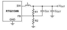
Figure 7. Feedback Loop with Feedforward Capacitor
