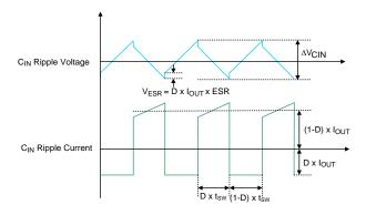
Figure 4. CIN Ripple Voltage and Ripple Current
