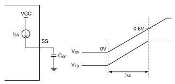
Figure 1. External Soft-Start Time Setting
