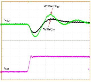
Figure 9. Load Transient Response with and without Feedforward Capactior
